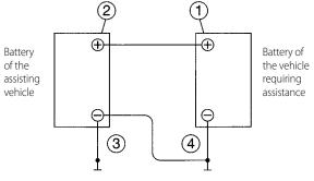
Now start the vehicle needing assistance for a maximum of 15 seconds. Do not start the assisting vehicle.
